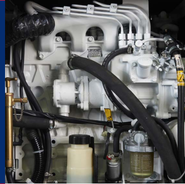
1800 rpm Kubota engine
