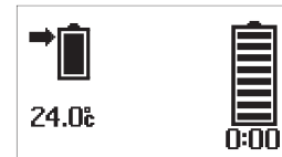
Full charging for operation complete
