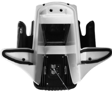
High-current connector plate in accumulator shaft
