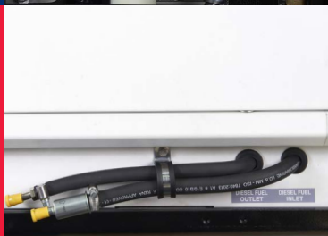
Input/Output fuel pipe
