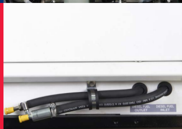
Input/Output fuel pipe
