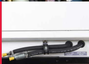
Input/Output fuel pipe
